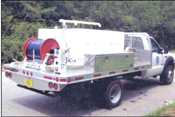
Harben truck mounted 300 to 700 gallon jetting packages can be fitted to a variety of diesel engine truck chassis up to 19,000 lb. GVW weight range.
